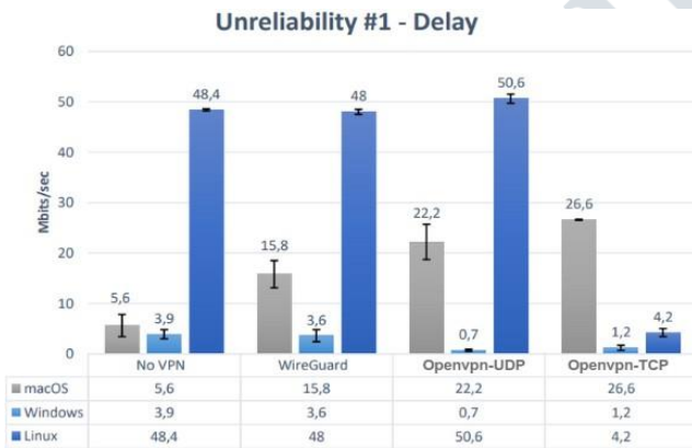
Figure 4. No VPN and VPN Performance under Unreliability #1 - Delay (Reference 1)
